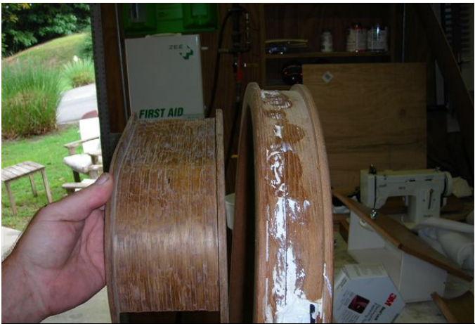
Thickness difference between new and old bulkheads.
