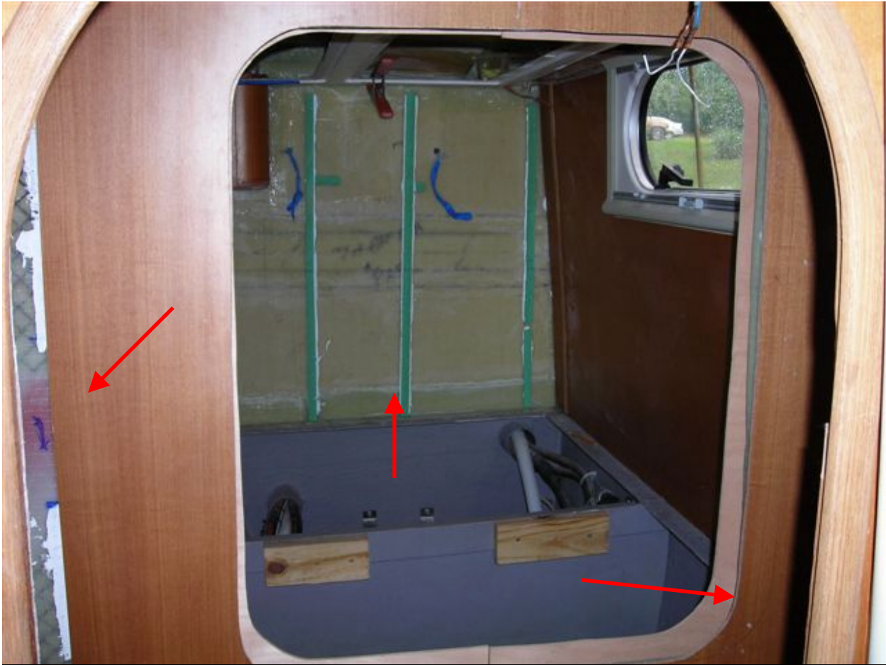
New or strengthened bulkheads indicated by arrows.
