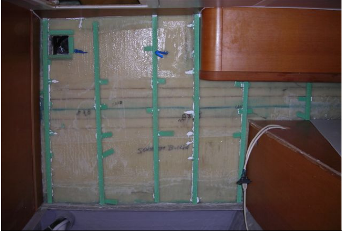
Newly reinforced aft cabin bulkheads ready for paneling.
