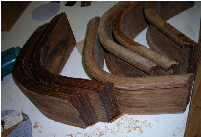
Custom-laminated corner trim in various stages of completeness.
