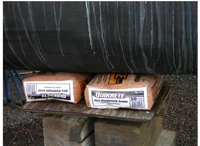
Sandbags required to prevent hull damage.
