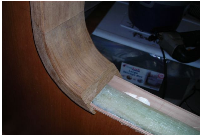
New bulkhead with trim temporarily fitted.
