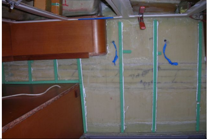
Newly reinforced aft cabin bulkheads ready for paneling.
