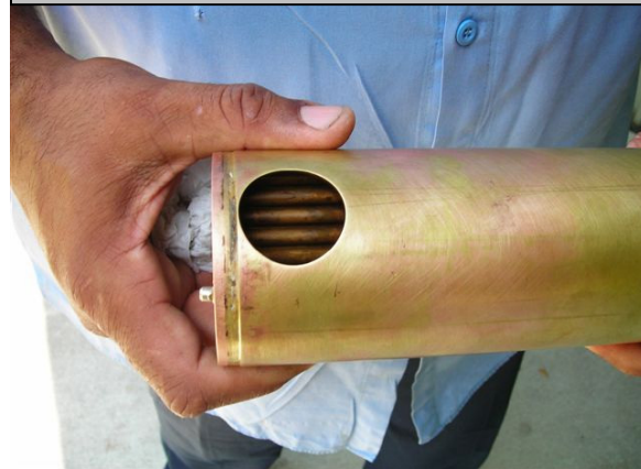
Heat exchanger after cleaning. Red hue indicates dezincification is taking place.
