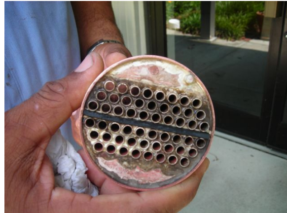
Heat exchanger after cleaning. Red hue indicates dezincification is taking place.
